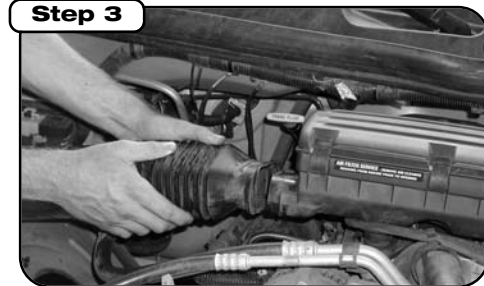
Remove air duct from resonator box and completely remove from engine compartment.
