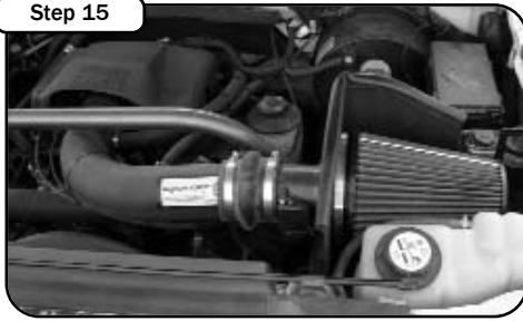
Place enclosed CARB EO sticker on a clean/smooth surface on or near the intake system. Your installation is now complete. Close hood slowly to verify hood clearance. Check and retighten connections and filter after a few hours of operation.
