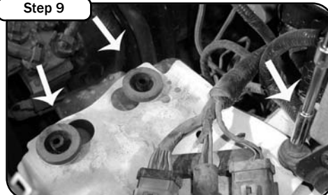
Remove the 8mm bolt that secures the cruise control (see arrow). Insert the plastic spacers into the rubber gromets. On the 04-05 models there is no cruise control bracket. A m6 screw and washer is provided.
