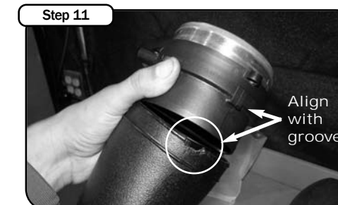
Step 11 Insert the MAF sensor into the aFe intake tube. Make sure to align the MAF sensor to the groove on the intake tube. This assembly requires a snug fit. If fit is too tight the tube can be heated with a hair dryer or heat gun to allow insertion.
