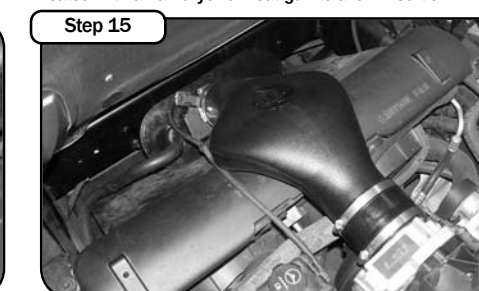
Step 15 Your installation is now complete. Make sure you tighten all clamps and check all electrical connections. Re-check periodically.
