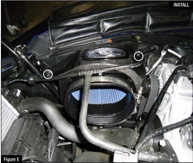
**Refer to Figure E for Step 7** Step 7: Install the aFe filter/housing assembly into the vehicle. Push it on the factory stud and secure it using the two factory 10 mm screws removed at step 4.
