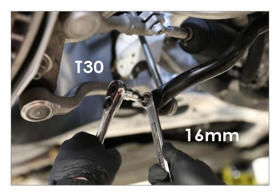
5F Undo the sway bar bushing brackets. (13mm socket)
