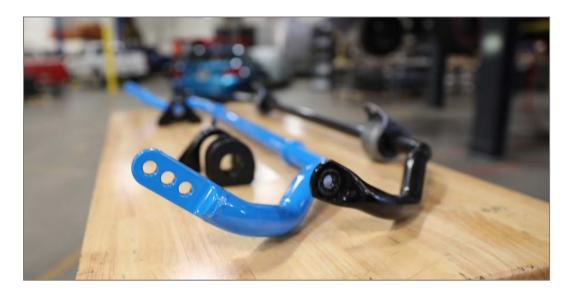
8F Grease the front bushings with the supplied silicone lube and install bushings onto the sway bar. The bushings should be positioned just outside of the centering rings.
