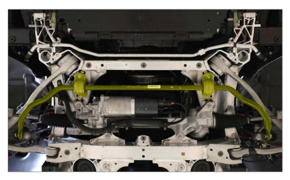
Disconnect the end links from the stock sway bar using a T30 torx socket for the stud and 16mm wrench for the nut.
