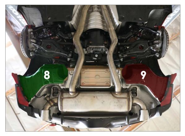
4R Remove the aluminum under brace (13mm & E14 torx sockets)
