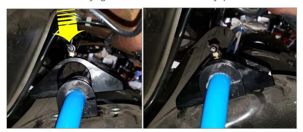
22R Reattach the end links to the sway ends reusing the factory nuts. The hole closest to the end is the soft setting. Settings get stiffer as you move away from the ends. (optional: apply thread locking compound to the end link thread)
