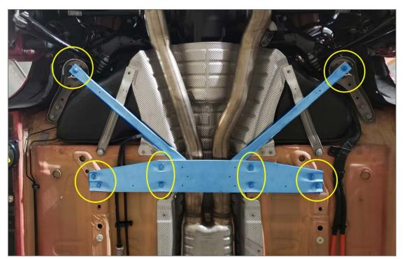
5R Remove the exhaust system starting just after the catalytic converter. Mounts and clamp can be removed with a 13mm socket.
