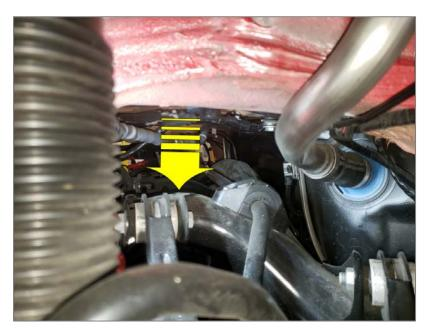
15R Disconnect the end links from the stock sway bar using a T30 torx socket for the stud and 16mm wrench for the nut.
