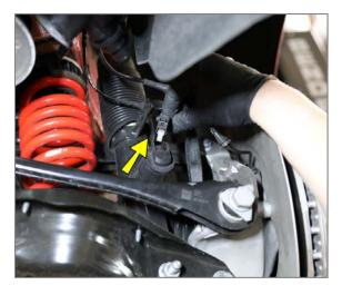
8R Disconnect the ground strap located on left side of diff. (10mm socket)
