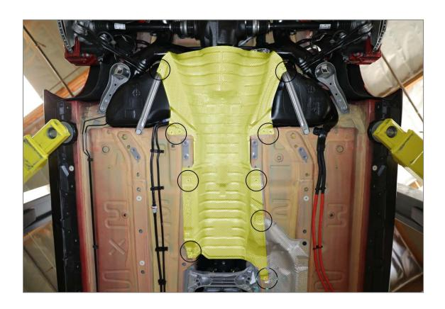
7R By hand, unclip the brake lines and ABS lines from their tab holders. Do not open any brake or abs lines. This allows some slack for the lines when you drop the subframe.
