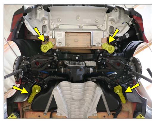
14R Lower the transmission jack slowly and check to make sure none of the lines are being tugged or pulled. If everything looks safe, lower the subframe about 4 inches or until there is enough room to sneak the rear sway bar out.
