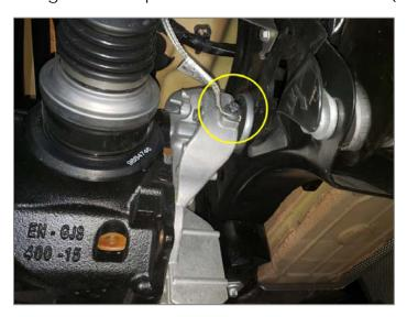
9R Disconnect the height sensor and all the line clips holding it to the subframe.
