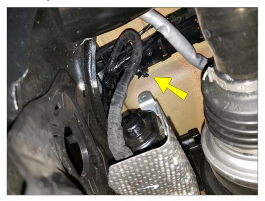
11R Unbolt the lower shock mounts. (18mm socket & wrench)
