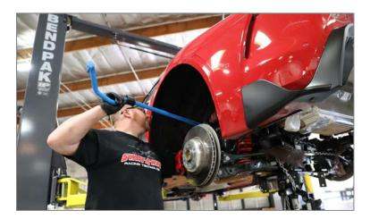
21R Slide the aFe Control bushing bracket onto the bushings and mate the sway bar assembly to the subframe. Make sure the grease fittings are pointed outward. Reuse the factory torx bolts to secure the brackets to the subframe. Fully tighten this hardware to factory specs.
