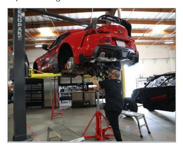
13R Next, unfasten the (4) main subframe mounts. Unbolt the hex bolts (16mm socket) from each of the four mounts first. Use an E18 torx socket and unfasten each of the (4) subframe main bolts.
