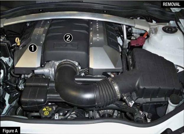
**Refer to Figure A for Step 1** Step 1: Remove the oil cap(1) and remove the engine cover(2). Reinstall the oil cap.
