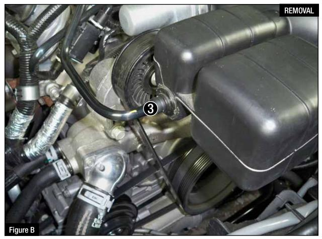
**Refer to Figure B for Step 2** Step 2: Disconnect the breather tube (3) from the intake tube.
