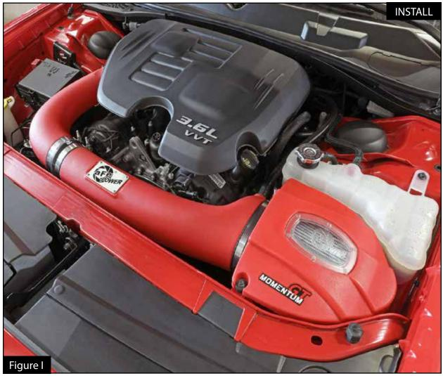
Refer to Figure I for Step 26 Step 26: Reinstall the engine cover.
