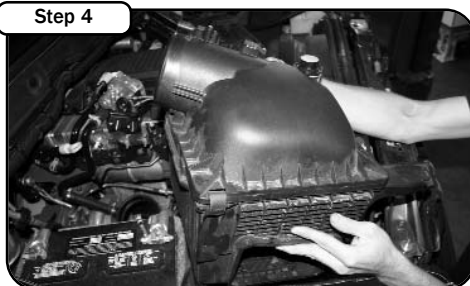
Loosen the 10mm nut at front of air box and remove. Carefully grab and pull out OE intake system from vehicle.
