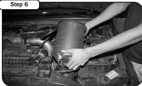
Step 6 Remove the inlet portion of the air box out of the engine bay.
