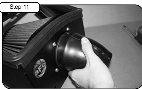
Step 11 Attach the coupler with the clamps provided to the filter adaptor. Do not tighten clamps.
