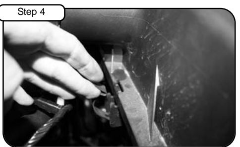
Step 4 Disengage the 3 clips which secure the upper portion of the airbox. Remove the center clip which is not used with the aFe intake.
