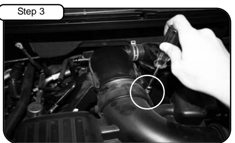
Step 3 Loosen the clamp on the throttle body tube using a 5/16" nut driver.
