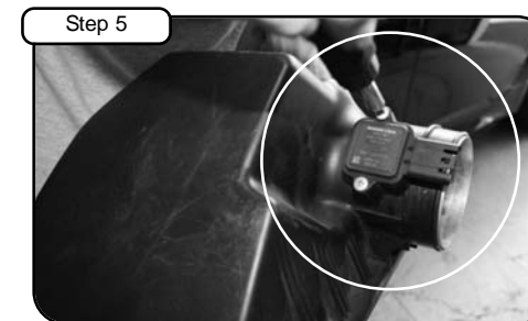
Carefully remove MAF sensor using T25 torx bit.
