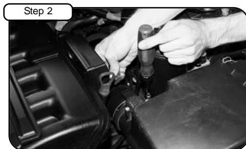
Disconnect MAF sensor. Loosen clamp on air box.
