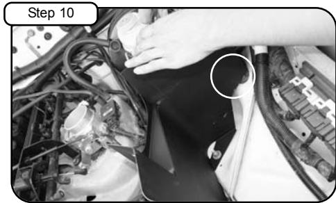
Step 10 Re-install nut from step 7 to secure back of housing tab to ECU bracket.
