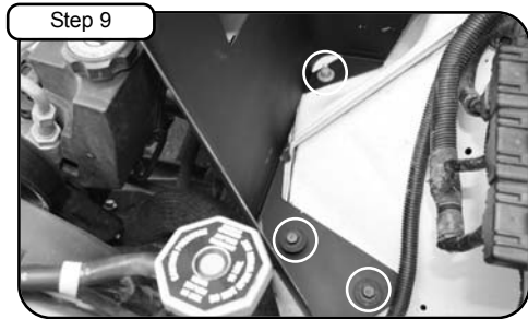
Step 9 Secure housing using the 2 bolts and 1 nut from step 5 and tighten using 12mm socket or wrench.
