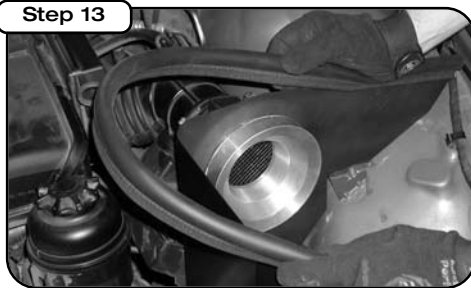
Install trim seal.
