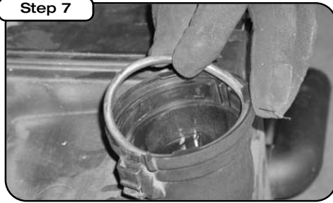
Carefully remove o-ring from stock air box.
