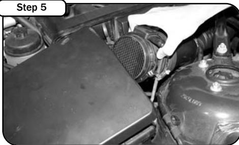
Remove MAF sensor from airbox. Make sure you do not damage the rubber gasket. Lift airbox out and remove from vehicle.
