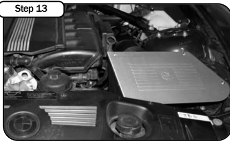
Place enclosed CARB EO sticker on a clean/smooth surface on or near the intake system. EO identification label is required in passing the Smog Check inspection. Your installation is now complete. Tighten all connections and clamps. Re-check after a few hours.
