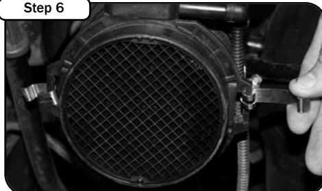
Install the two spring clips to the MAF sensor.
