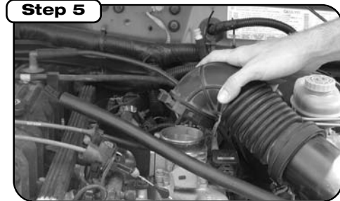
Loosen clamp at throttle body and remove.
