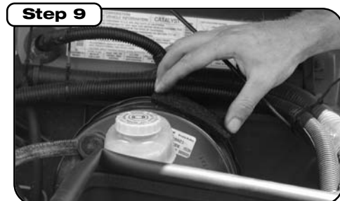
Looking straight at brake booster place center of isolation pad at 1 o'clock.
