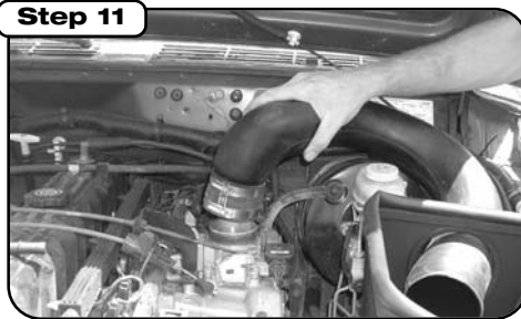
Slip coupler over throttle body.
