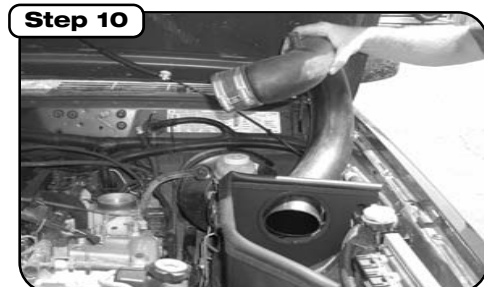
Attach coupler to intake at throttle body end. Then slide intake tube through filter housing starting with filter end of tube.
