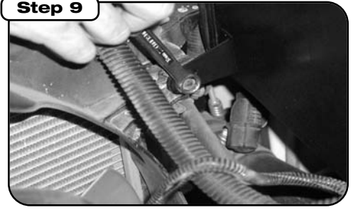
Using the bolt removed from the fan shroud earlier, secure the heat shield to the shroud using the tab extending from the heat shield, do not fully tighten.
