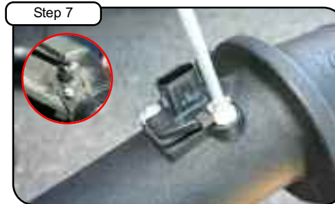
Step 7 With T-20 torx bit remove MAF sensor and ( with gasket, nylon spacers and screws provided ) install into new tube. Make sure gasket and nylon spacers are between sensor and tube.
