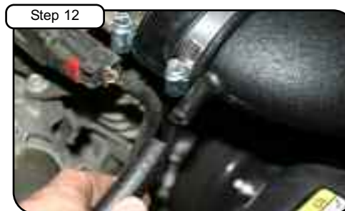
Step 12 Install new 3/8" provided to valve cover side and new tube side.
