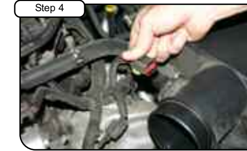
Step 4 Disconnect MAF sensor harness.
