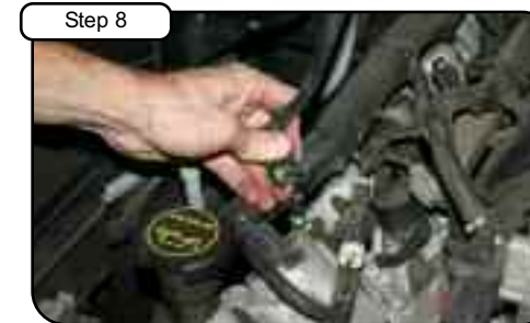
Step 8 Remove factory crank case line from engine.
