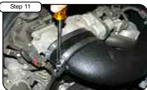
Step 11 Tighten clamps with 5/16" nut driver.
