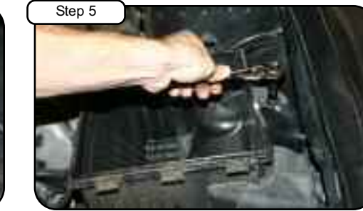
Step 5 With 10mm socket or wrench loosen the 2 screws holding in OE air box. Lift up and remove OE air box out of vehicle.
