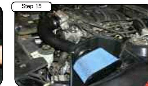
Step 15 Your installation is now complete. Please check all bolts and clamps periodically. Re-tighten if necessary. Thank you for choosing aFe! Place enclosed CARB EO sticker on a clean/smooth surface on or near the device. EO identification label is required in passing the smog check inspection.
