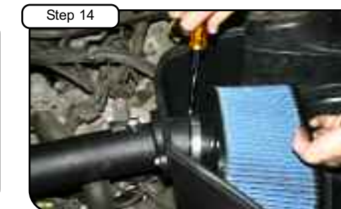
Step 14 Install air filter and tighten using 5/16" nut driver.
