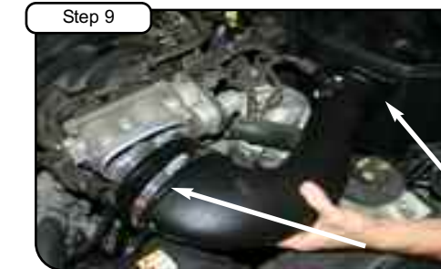
Step 9 Install coupler with clamps to tube. Install tube to outside of housing and position coupler on to throttle body.
