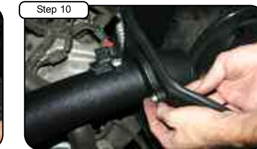
Step 10 Install screws/nuts and washer provided to mount tube to housing. Tighten using 10mm socket or wrench.
