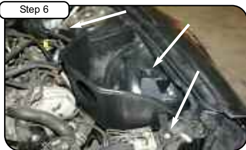
Step 6 With OE screws removed from step 5, install new aFe housing to vehicle. Tighten using 10mm socket or wrench.
