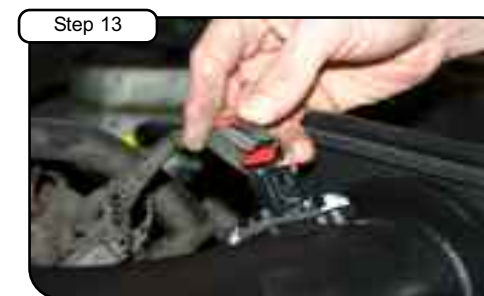
Step 13 Reconnect MAF sensor harness.
