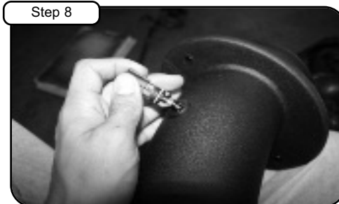
Install supplied grommet into tube. Carefully place air temp sensor into new aFe intake tube .
