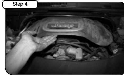
Carefully remove engine cover, remove oil cap first and gently pull up and forward.
