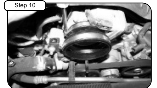
Place the reducer coupler onto the throttle body with supplied clamps. Tighten down the clamp at throttle body only.
