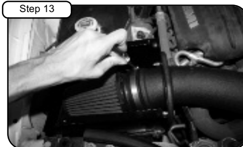
Place high flow aFe filter onto tube. Tighten using 5/16" nut driver. Gently place cover onto housing using the 4 button head screws. Tighten using 5/32" allen wrench.
