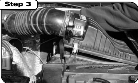
Loosen clamp from stock intake tube (at engine side), disconnect plug to filter minder and undo clips to remove top of OE air box.
