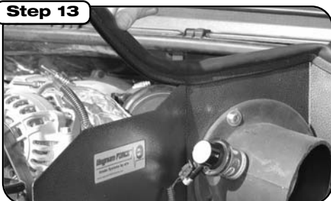
Install trim seal on housing.
