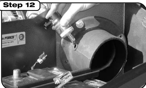
Place grommet into hole of intake tube. Insert filter minder into location and reconnect wire.
