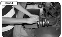
Install intake filter into housing. Re-connect the MAF sensor. Your Stage 1 installation is now complete. Make sure you tighten all clamps and check all electrical connections. Re-check periodically. Continue onto steps 11-13 to install Stage 2.
