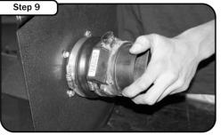
Slide the MAF sensor, clamps (#072 and #064), and reducer coupler (05-00020) on the air filter adaptor. Do not tighten the clamps at this time.
