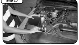
Place the rubber trim seal along edges of the housing. Bolt the housing to the engine bay using the factor bolts removed in Step 6. If installing stage 1 kit reconnect factory tube to MAF sensor.
