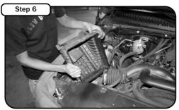
Grab the lower portion of the airbox then lift up and out. The box is secured with rubber gromets.
