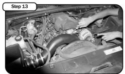
Place reducer coupling (05-00020) with clamps (#60) on throttle body and the hump coupler (05-00565) with clamps (#064) on the MAF sensor. Install intake tube. Tighten and secure all hose clamps. Botate fan to make sure there is sufficient clearance between the intake tube and the fan-
