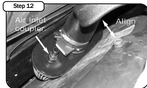
Step 12 Insert the air hose inlet coupler into the air filter. Sit the intake into position aligning the two rubber grommets with the dimples on the aFe intake tube.
