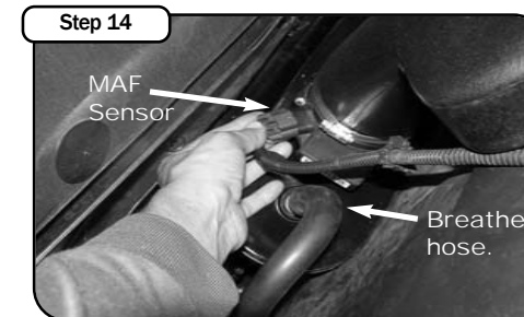
Step 14 Reconnect the MAF sensor and air inlet hose to the air filter.
