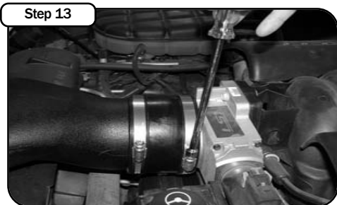
Step 13 Secure the coupler onto the throttle body and secure in position.
