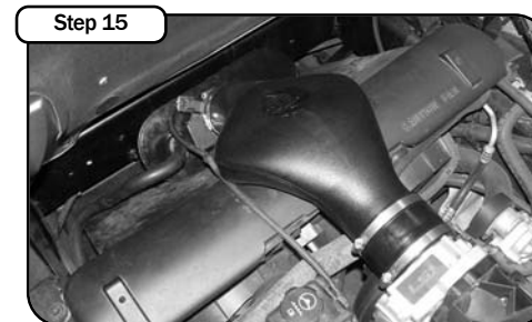
Step 15 Place enclosed CARB EO sticker on a clean/smooth surface on or near the intake system. EO identification label is required in passing the Smog Check inspection. Your installation is now complete. Make sure you tighten all clamps and check all electrical connections. Re-check periodically.
