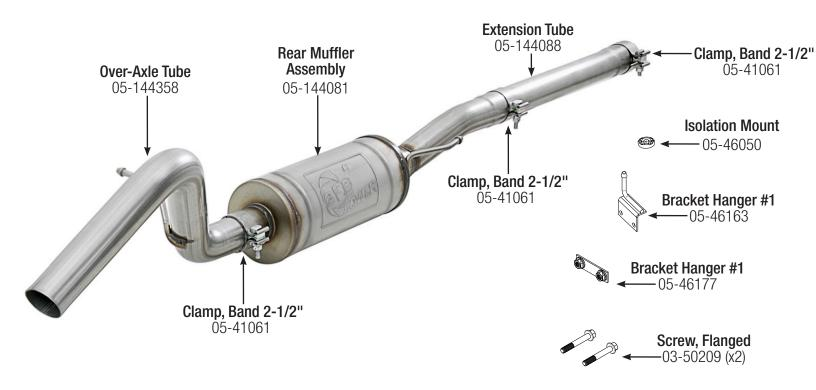
Professional installation is highly recommended. (Read instructions prior to installation) To, work properly with the vehicle. **Make sure to always have at least (2) stands or jacks on hand to support the removal of 0E system. As, well as for the installation of aFe system. Any Removal of rubber isolation mounts may require using a spray lubricant such as WD40 and a pry bar.**
