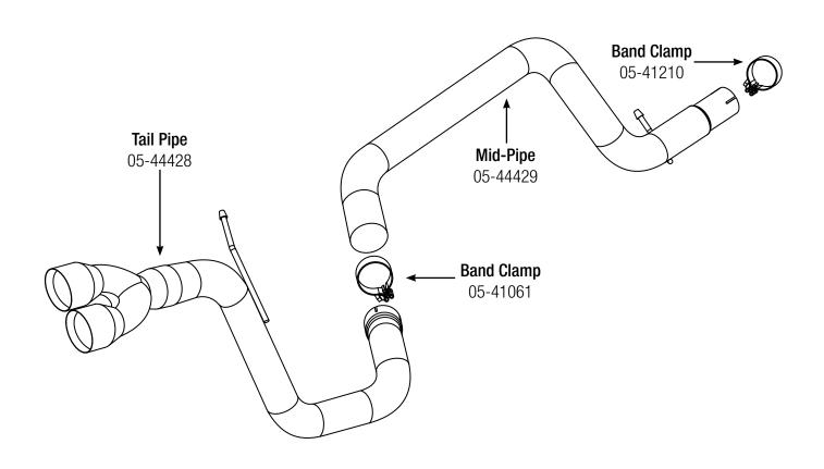
Step 1: (Read Instructions prior to installation) Remove your stock exhaust from the rear of your vehicle working your way forward. It is recommended to not fully tighten the clamps until the entire system has been installed.
