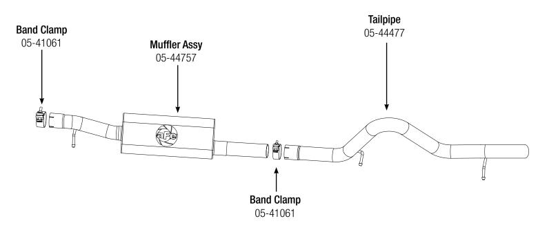
**Step 1:** (Read Instructions prior to installation) <u>Remove your stock exhaust</u> from the rear of your truck working your way forward. Take caution not to damage the factory isolation mounts as they will be reused. It may be helpful to lubricate the isolation mounts prior to disassembly. It is recommended to not fully tighten the clamps until the entire system has been installed.
