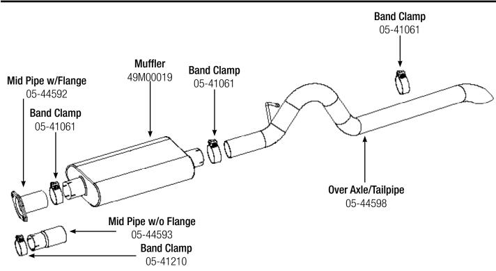
**Step 1: (Read Instructions prior to installation)** <u>Remove your stock exhaust</u> from the rear of your truck working your way forward. Take caution not to damage the factory isolation mounts as they will be reused. It may be helpful to lubricate the isolation mounts prior to disassembly. **It is recommended to not fully tighten the clamps until the entire system has been installed.**
