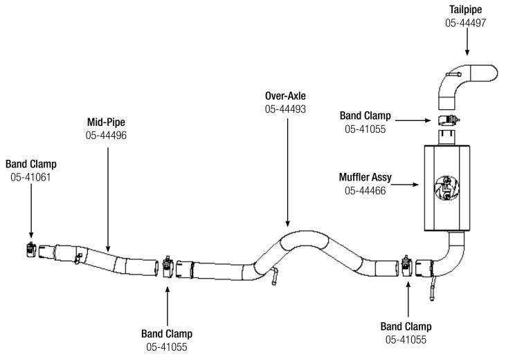
**Step 1:** (Read Instructions prior to installation) <u>Remove your stock exhaust</u> from the rear of your truck working your way forward. Take caution not to damage the factory isolation mounts as they will be reused. It may be helpful to lubricate the isolation mounts prior to disassembly. It is recommended to not fully tighten the clamps until the entire system has been installed.
