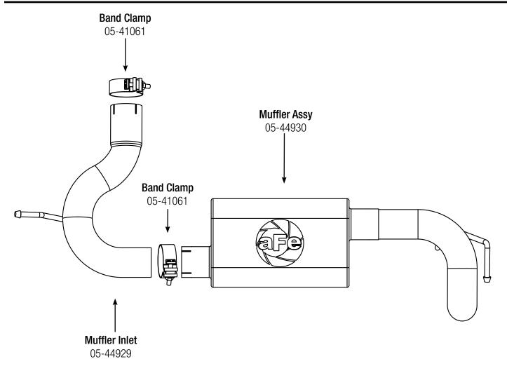
**Step 1:** (Read Instructions prior to installation) Remove your stock exhaust from the rear of your truck working your way forward. Take caution not to damage the factory isolation mounts as they will be reused. It may be helpful to lubricate the isolation mounts prior to disassembly. It is recommended to not fully tighten the clamps until the entire system has been installed.
