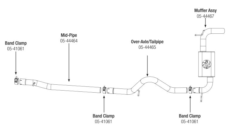
**Step 1:** (Read Instructions prior to installation) Remove your stock exhaust from the rear of your truck working your way forward. Take caution not to damage the factory isolation mounts as they will be reused. It may be helpful to lubricate the isolation mounts prior to disassembly. It is recommended to not fully tighten the clamps until the entire system has been installed.
