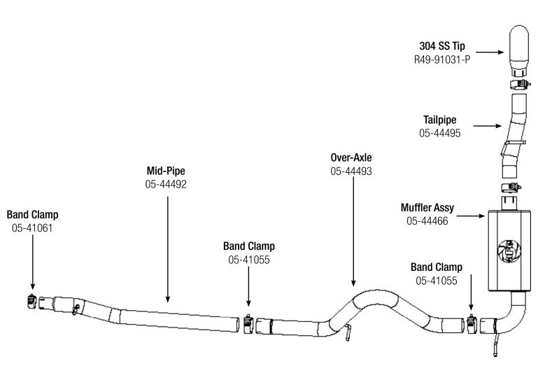
**Step 1:** (Read Instructions prior to installation) Remove your stock exhaust from the rear of your truck working your way forward. Take caution not to damage the factory isolation mounts as they will be reused. It may be helpful to lubricate the isolation mounts prior to disassembly. It is recommended to not fully tighten the clamps until the entire system has been installed.
