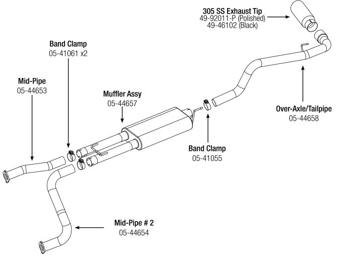
**Step 1:** (Read Instructions prior to installation) Remove your stock exhaust up to the catalytic converter from the rear of your truck working your way forward. Take caution not to damage the factory hardware and isolation mounts as they will be reused. It is recommended to not fully tighten the clamps until the entire system has been installed.
