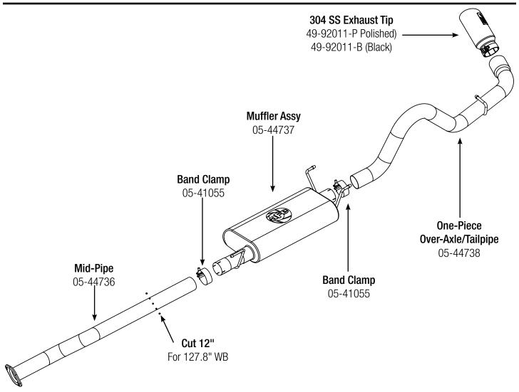
**Step 1: (Read Instructions prior to installation)** Remove your stock exhaust up to the catalytic converter from the rear of your truck working your way forward. Take caution not to damage the factory hardware and isolation mounts as they will be reused.
