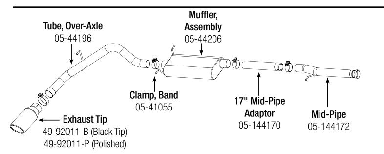
Caution: Allow time for your vehicle to cool down prior to installation. When working on or under your vehicle proceed with caution. Exhaust systems reach high temperatures and may cause serious burns. Wear protective safety equipment; eye goggles and gloves to ensure a safe installation. <u>aFe recommends</u> professional installation on our products.
