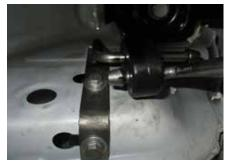
**Step 6:** Install the Rear tube using provided 3" band clamp and provided isolation mount. **Step 7:** Align exhaust system and tighten all band clamps, re-install
