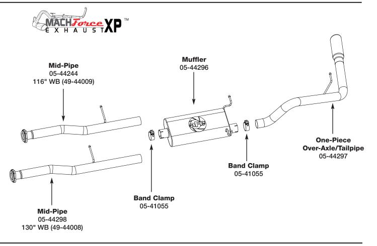
Step 1: (Read Instructions prior to installation) <u>Remove your stock exhaust</u> up to the catalytic converter from the rear of your truck working your way forward. Take caution not to damage the factory isolation mounts as they will be reused. This system is best installed with a chassis lift with axles extended for clearance. It is recommended to not fully tighten the clamps until the entire system has been installed.
