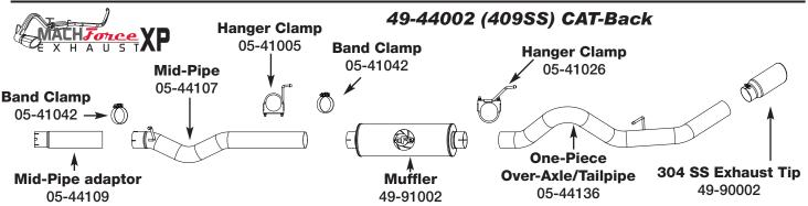
**Step 1:** (Read Instructions prior to installation) Remove your stock exhaust up to the cataytic converter from the rear of your truck working your way forward. It may be necessary to cut the pipes if the slip joints are stuck. Take caution not to damage the factory isolation mounts as they will be reused.. It is recommended to not fully tighten the clamps until the entire system has been installed.
