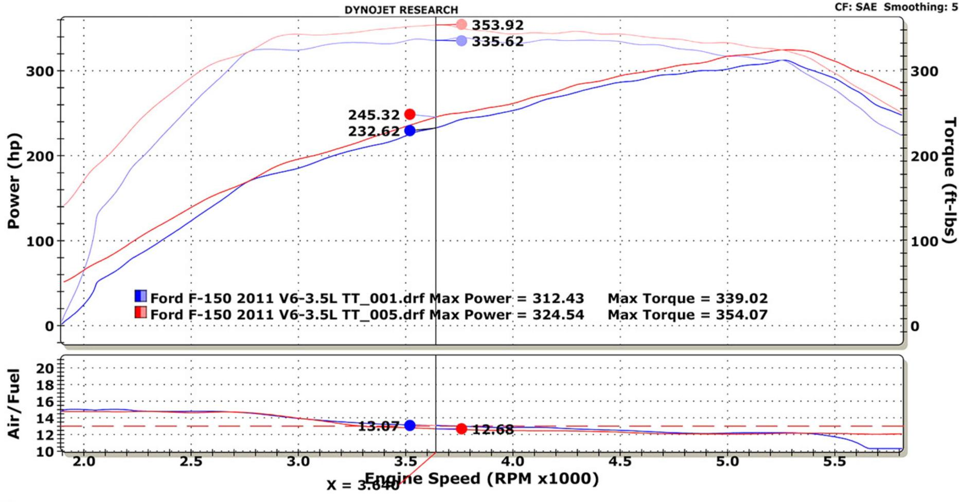
Ford F-150 2011 V6-3.5L TT\_001.drf - 4/15/2015 10:59:37 AM Run Type: RO Run Conditions: 78.00 °F, 29.04 in-Hg, Humidity: 6%, SAE: 1.01 Base Line
