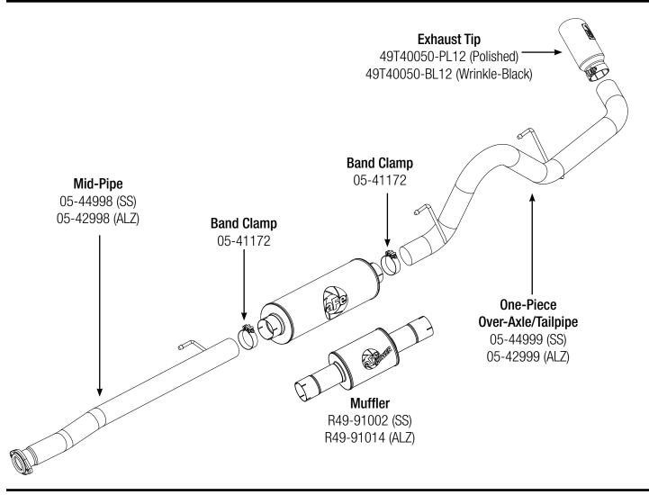
Step 1: (Read Instructions prior to installation) Remove your stock exhaust up to the catalytic converter from the rear of your truck
