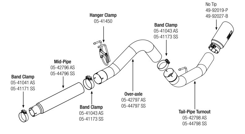
Step 1: (Read Instructions prior to installation) Loosen mounting flange at rear of particulate filter before muffler. Remove the stock exhaust from the rear of the truck working your way forward. Take caution not to damage the factory isolation mounts and gasket as they will be reused. It is recommended to not fully tighten the clamps until the entire system has been installed.
