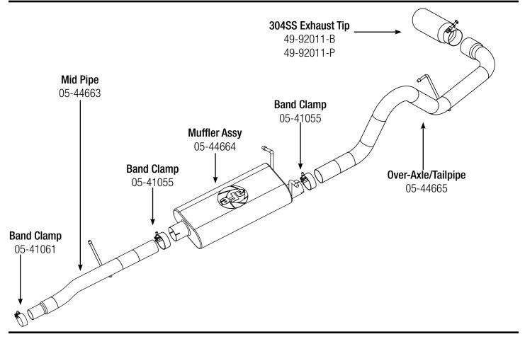
**Step 1: (Read Instructions prior to installation)** Remove your stock exhaust up to the catalytic converter from the rear of your truck working your way forward. Take caution not to damage the factory band clamp and isolation mounts as they will be reused.. It is recommended to not fully tighten the clamps until the entire system has been installed.
