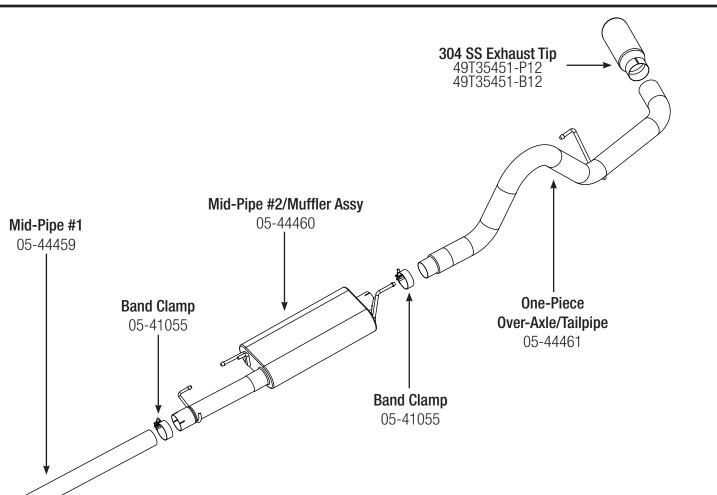
**Step 1: (Read Instructions prior to installation)** Remove your stock exhaust up to the catalytic converter from the rear of your truck working your way forward. Take caution not to damage the factory hardware and isolation mounts as they will be reused.
