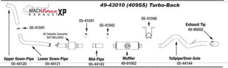
1: (Read Instructions prior to installation) Remove your stock exhaust from the rear of your truck working your way forward. Take caution not to damage the factory isolation mounts. If you want to remove the OE downpipe in one piece or without cutting, you must remove the transmission cross member and disconnect the dip-stick tube & sway bar end links. It is recommended to not fully tighten the clamps until the entire system has been installed.
