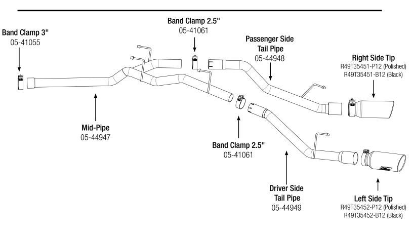
Step 1: (Read Instructions prior to installation) Loosen mounting flange at rear of particulate filter before muffler. Remove the stock exhaust from the rear of the truck working your way forward. Take caution not to damage the factory isolation mounts and gasket as they will be reused. It is recommended to not fully tighten the clamps until the entire system has been inställed.
