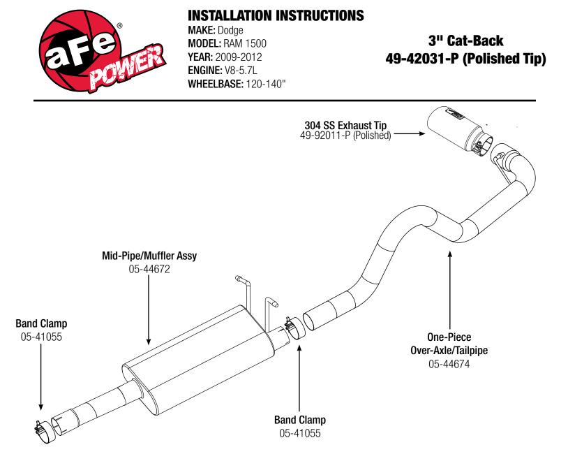
Step 1: (Read Instructions prior to installation) <u>Remove your stock exhaust</u> from the rear of your truck working your way forward. It may be necessary to cut the pipes if the slip joints are stuck. Do not cut the pipe after the cat. You will be using this slip connection. Take caution not to damage the factory isolation mounts, as they will be reused. It is recommended to not fully tighten the clamps until the entire system is installed.
