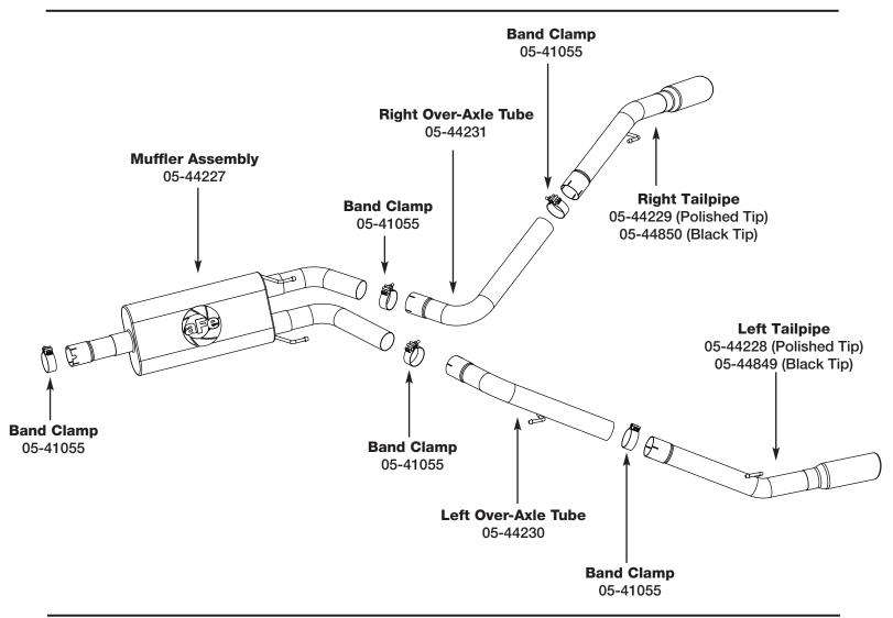
Step 1: (Read Instructions prior to installation) Remove your stock exhaust from the rear of your truck working your way forward. Disconnect the ground strap from chassis to muffler and save for re-use later. Also take caution not to damage the factory isolation mounts as they will be reused. It is recommended to not fully tighten the clamps until the entire system has been installed.
