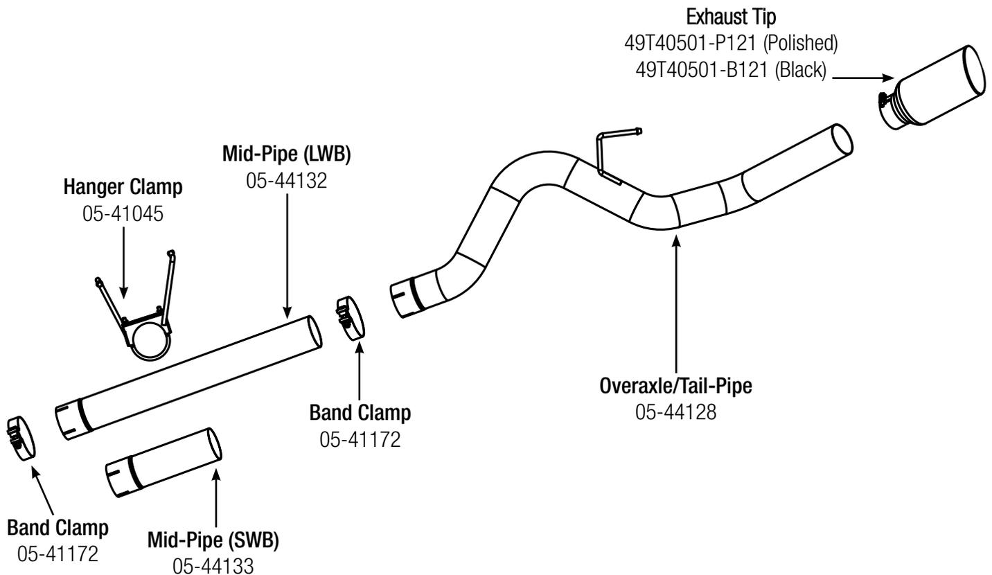
**Step 1: (Read Instructions prior to installation)** Loosen band clamp at rear of particulate filter before muffler. Remove the stock exhaust from the rear of the truck working your way forward. Take caution not to damage the factory isolation mounts as they will be reused. **It is recommended to not fully tighten the clamps until the entire system has been installed.**
