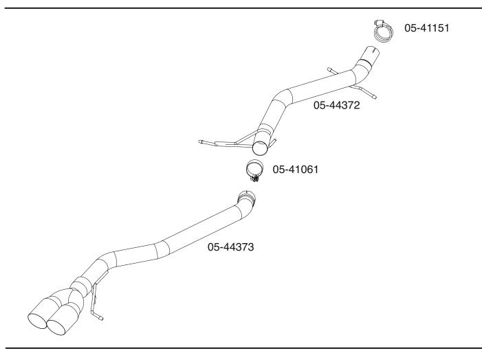
**Step 1:** (Read Instructions prior to installation) Remove your stock exhaust from the rear of your vehicle working your way forward. It will be necessary to cut the pipe to clear the rear axle. Do not cut the pipe after the cat; you will be using this slip connection.
