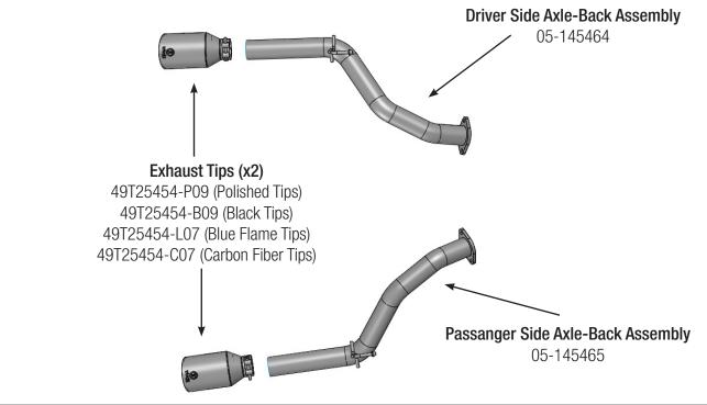
Professional installation is highly recommended. (Read instructions prior to installation). Make sure to always have at least (2) stands or jacks on hand to support the removal of OE system. Also for the installation of aFe system. Any Removal of rubber isolation mounts may require using a spray lubricant such as WD40 and a pry bar.
