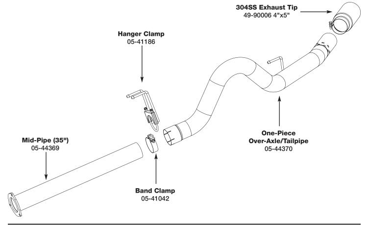
Step 1: (Read Instructions prior to installation) Remove your stock exhaust from the rear of your truck working your way forward. The spare tire and heat shield will need to be removed for exhaust replacement. Take caution not to damage the factory isolation mounts as they will be reused. It is recommended to not fully tighten the clamps until the entire system has been installed.
