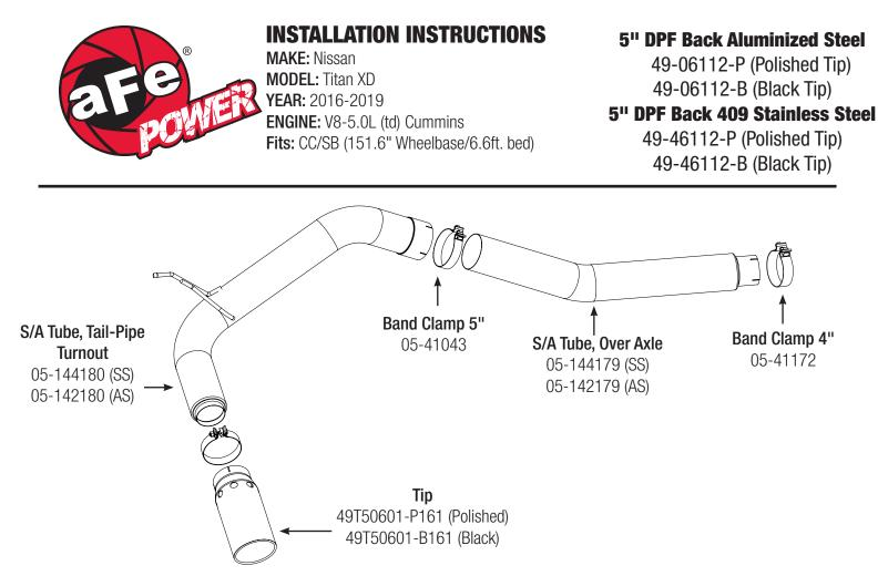
Professional installation is highly recommended. (Read instructions prior to installation). Make sure to always have at least (2) stands or jacks on hand to support the removal of OE system. Also for the installation of aFe system. Any Removal of rubber isolation mounts may require using a spray lubricant such as WD40 and a pry bar.
