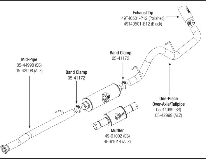
**Step 1: (Read Instructions prior to installation)** Remove your stock exhaust up to the catalytic converter from the rear of your truck working your way forward. Take caution not to damage the factory hardware and isolation mounts as they will be reused. **It is recommended to not fully tighten the clamps until the entire system has been installed.**
